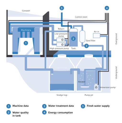
Detailed cross-section of a water treatment system (in this case AquaPur Modular). WashTec supplies the entire machinery.
